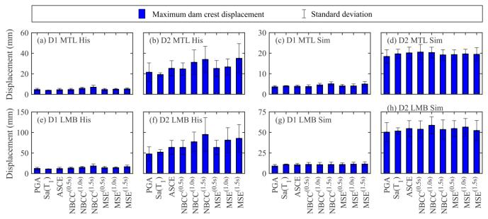
Figure 4 Mean value of maximum crest displacement of studied dams, computed using ground motion suites scaled according to different methods, from historical database as well as simulated database
