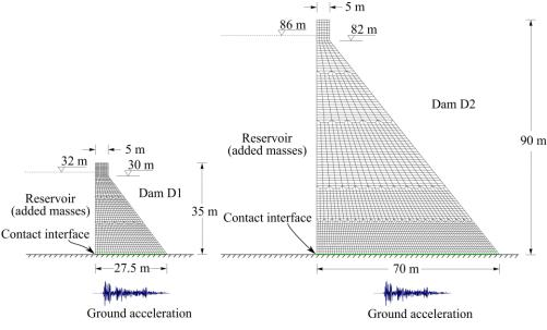
Figure 1 Geometry and finite elements model of D1 and D2 dam
