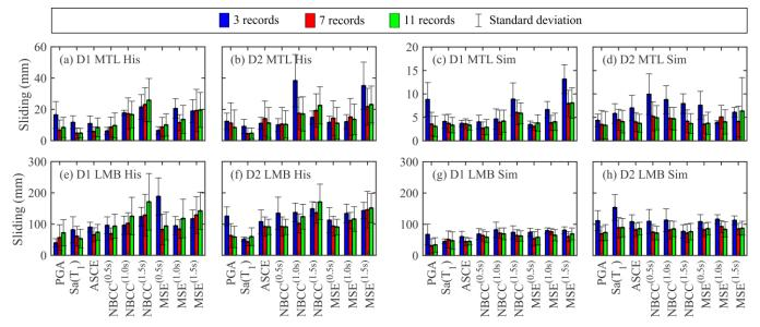
Figure 7 Comparison of sliding displacement estimated with maximum response of groups with 3 records, the mean response of groups with 7 records and groups with 11 records. Friction angle is taken as  $\phi = 45^{\circ}$ .
