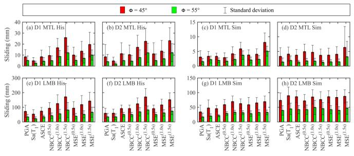
Figure 6 Mean residual sliding displacements of studied dams considering different friction angles \phi, computed using ground motion suites scaled according to different methods, from historical database as well as simulated database
