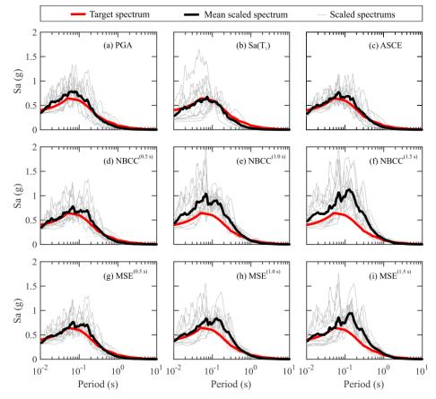
Figure 3 Mean scaled spectrum and individual scaled spectrum produced by different scaling methods for D1 dam in Montreal using historical ground motions
