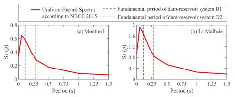
Figure 2 Target spectra of Montreal and La Malbaie for soil type A
