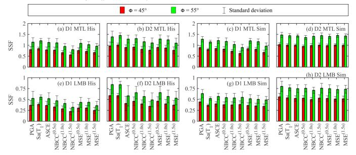
Figure 5 Mean value of SSF of studied dams considering different friction angles  $\phi$ , computed using ground motion suites scaled according to different methods, from historical database as well as simulated database
